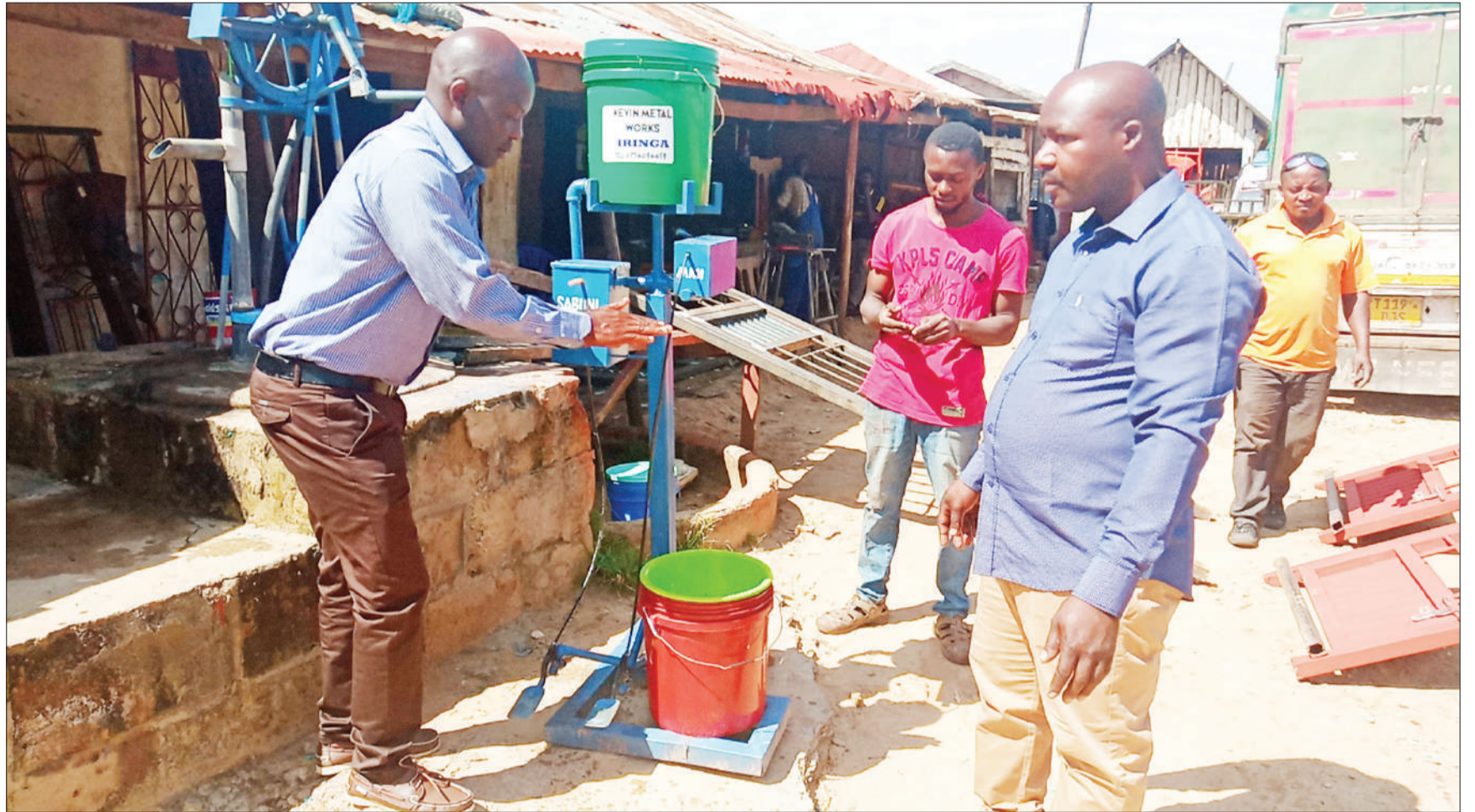
Kevin Mwanyika (L) of Kihesa in Iringa Region, who makes machines facilitating the washing of hands, demonstrates to a would-be customer yesterday how to use the 150,000/-a-piece tools without actually touching them – as a precaution against COVID-19 infections. He said a 20-litre bucket of water can serve up to 200 people at a go. Photo: Correspondent Francis Godwin
