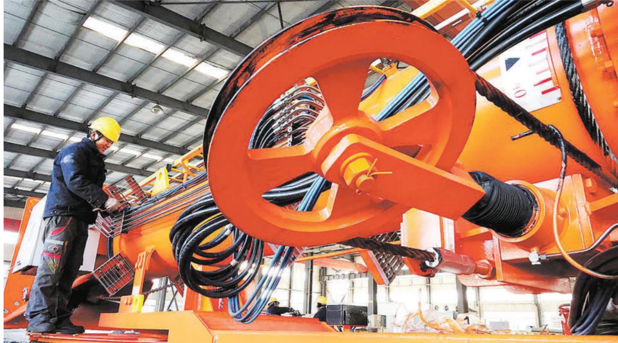
A worker assembles a liquid loading arm at an equipment manufacturing plant in Lianyungang, Jiangsu province.
