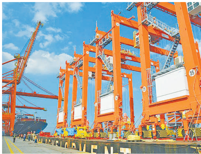
Hybrid Rubber-Tyred Gantry (RTG)
