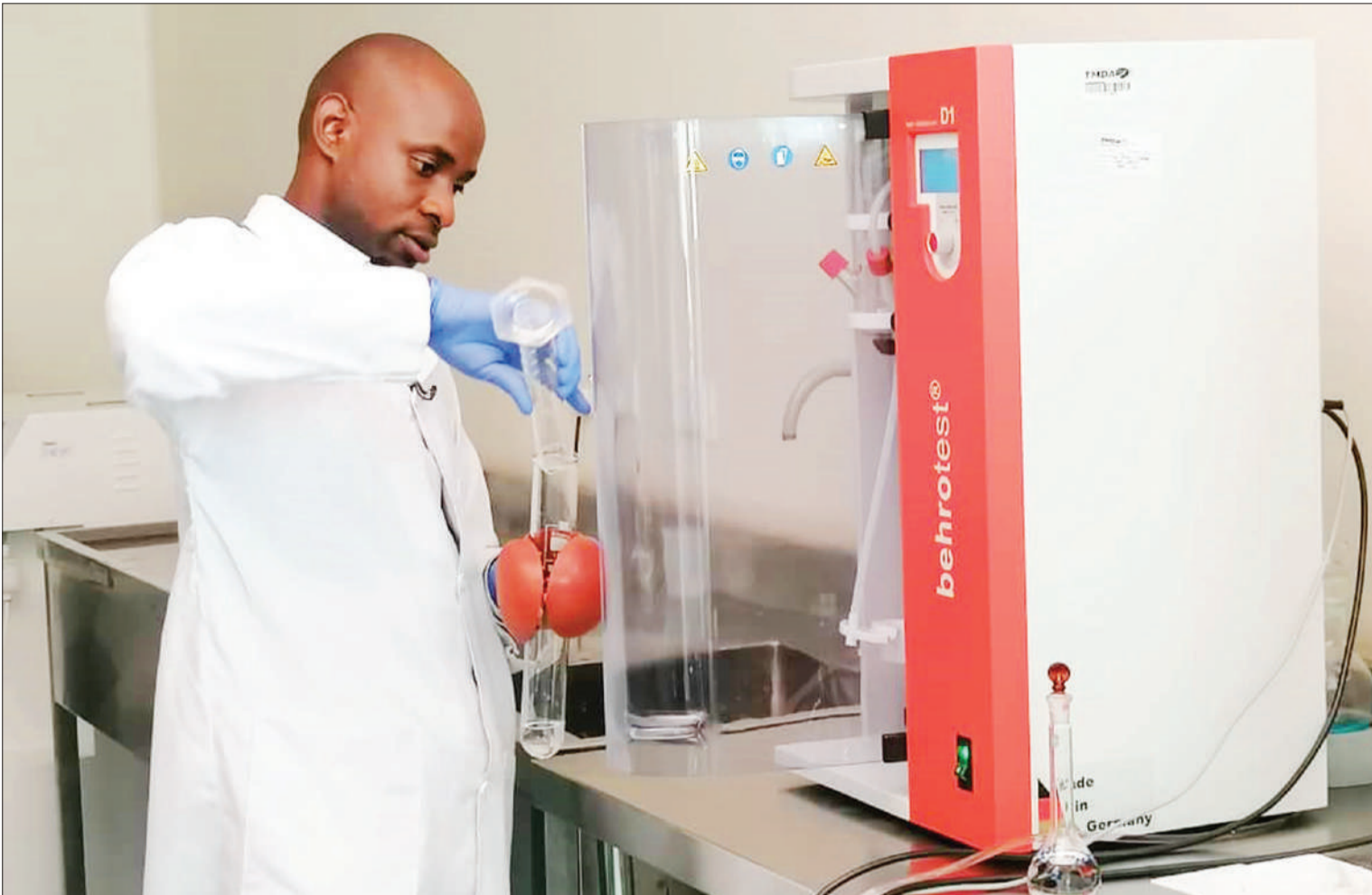
Jovinary Rwezahura, an analyst with the Tanzania Medicines and Medical Devices Authority's zonal laboratory in Mwanza city, pictured yesterday checking the level of alcohol in antiseptics using special high-speed machine known as steam distillation unit. Photo: Correspondent Devota Mwachanga
