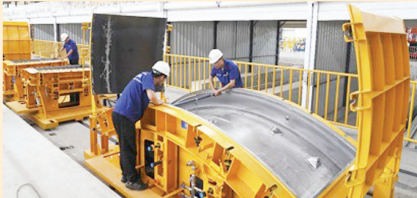
Technicians examine the precision of subway tunnel segment mold at a green intelligent building industrial base of China Railway Construction Corporation Limited (CRCC) in Beibei district, southwest China's Chongqing municipality, April 25, 2022. The industrial base uses modular prefabricated components and assembles them at construction sites, shifting tasks that were formerly performed on construction sites to factories. File photo
