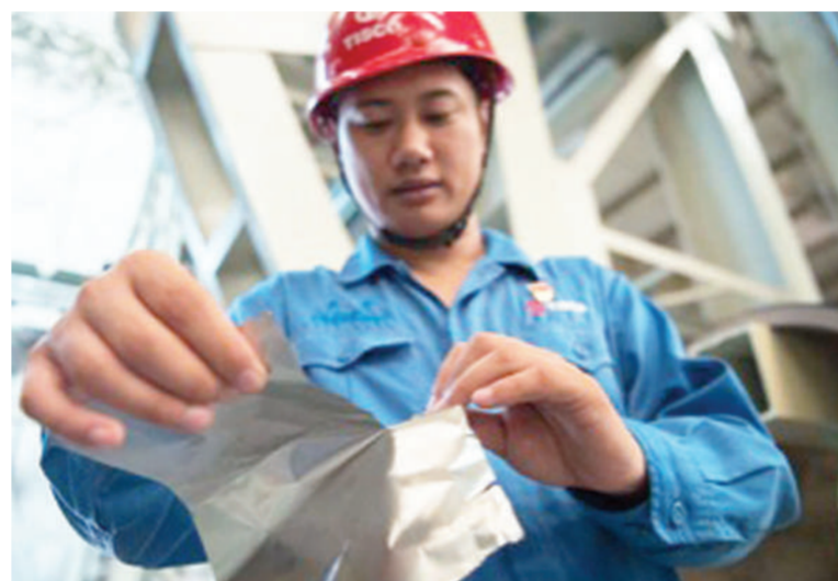
Liao Xi, a technician with the Shanxi Taigang Stainless Steel Precision Strip Co., Ltd., a subsidiary of Chinese steelmaker China Baowu, demonstrates the company's extremely thin stainless steel foil, which is known as "hand-torn steel" as it can be easily ripped by hand. File Photo
