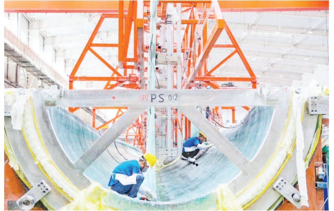
Wind turbine blades are manufactured in a workshop of a new material company in Changji Hui autonomous prefecture, northwest China's Xinjiang Uygur autonomous region. (People's Daily Online/He Long)
