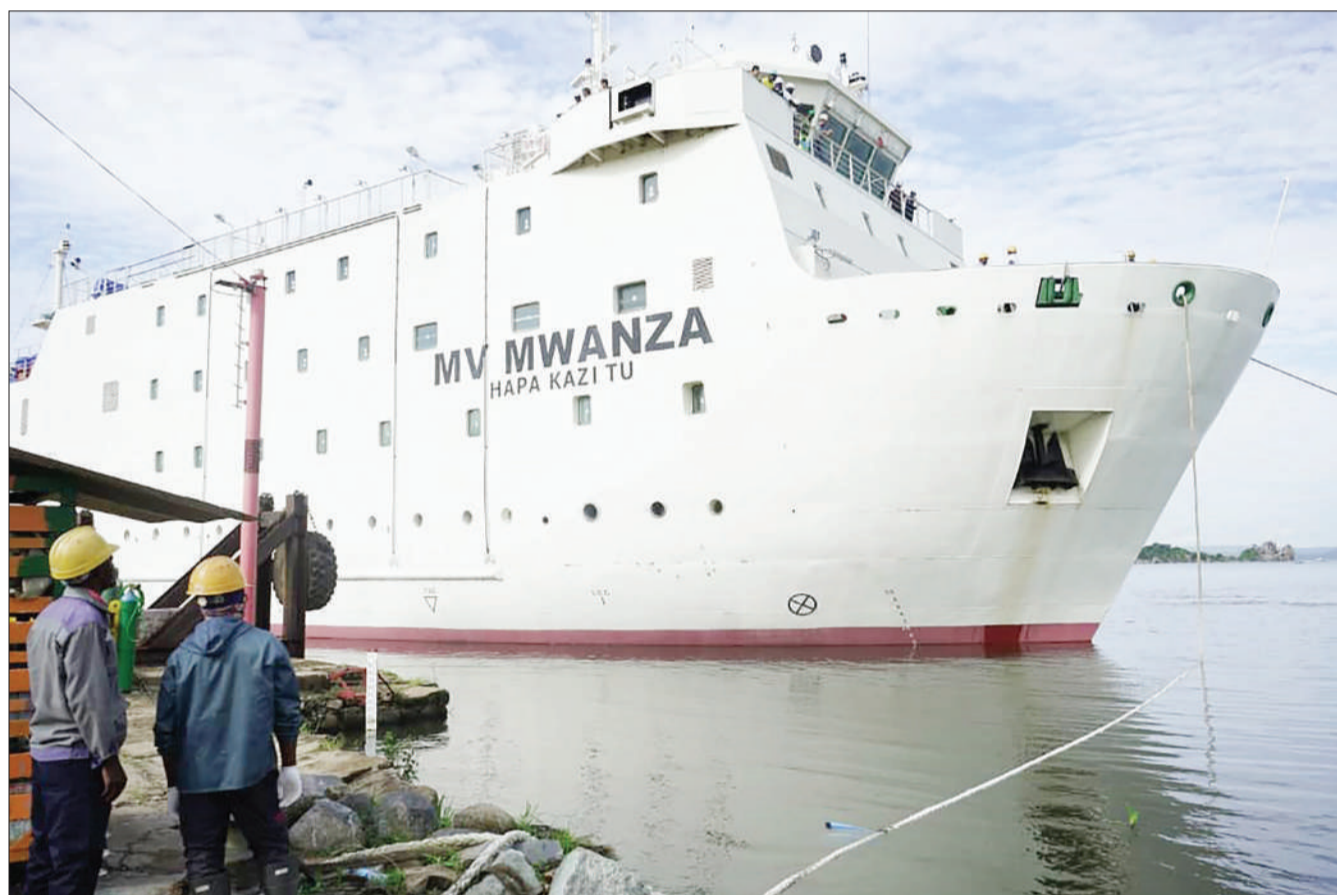
MV Mwanza 'Hapa Kazi Tu', whose construction was completed recently, captured on the third consecutive day of test-runs close to the Mwanza shores of Lake Victoria yesterday. Sources say the 92.6-metre-long Tanzanian vessel has capacity for 1,200 passengers, 400 tonnes of cargo, 20 vehicles and three trucks. Photo: Correspondent Vitus Audax
