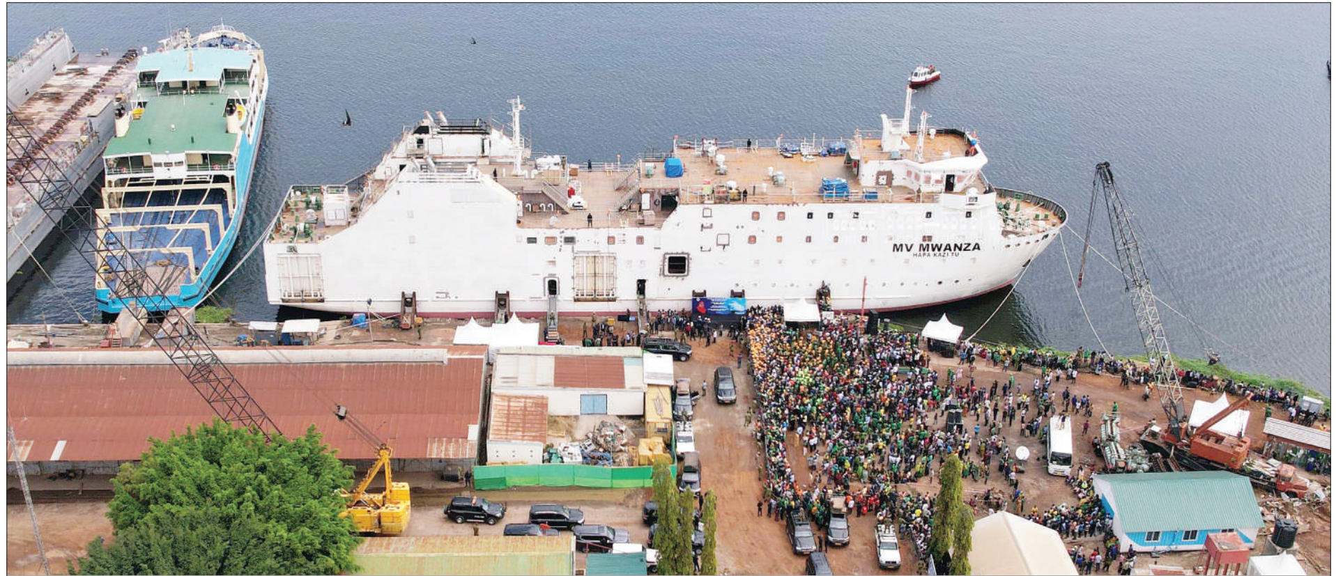
A view of MV Mwanza 'Hapa Kazi Tu', a passenger and cargo ship now in the final stages of construction at the Mwanza South Port, as captured yesterday. The vessel, meant to ferry 1,200 passengers, 400 tonnes of cargo and 20 vehicles, is being built by South Korean contractors in collaboration with Tanzanian Navy engineers. President Samia Suluhu Hassan, currently on a tour of Mwanza Region, inspected it yesterday. Photo: State House
