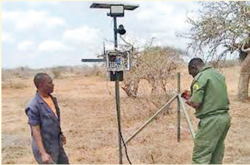
The NdovuCare device consists of a GSM card, a motion detector, a warning light and a siren and can detect an elephant at a radius of 180 metres. It offers a solution to human-wildlife conflict.
