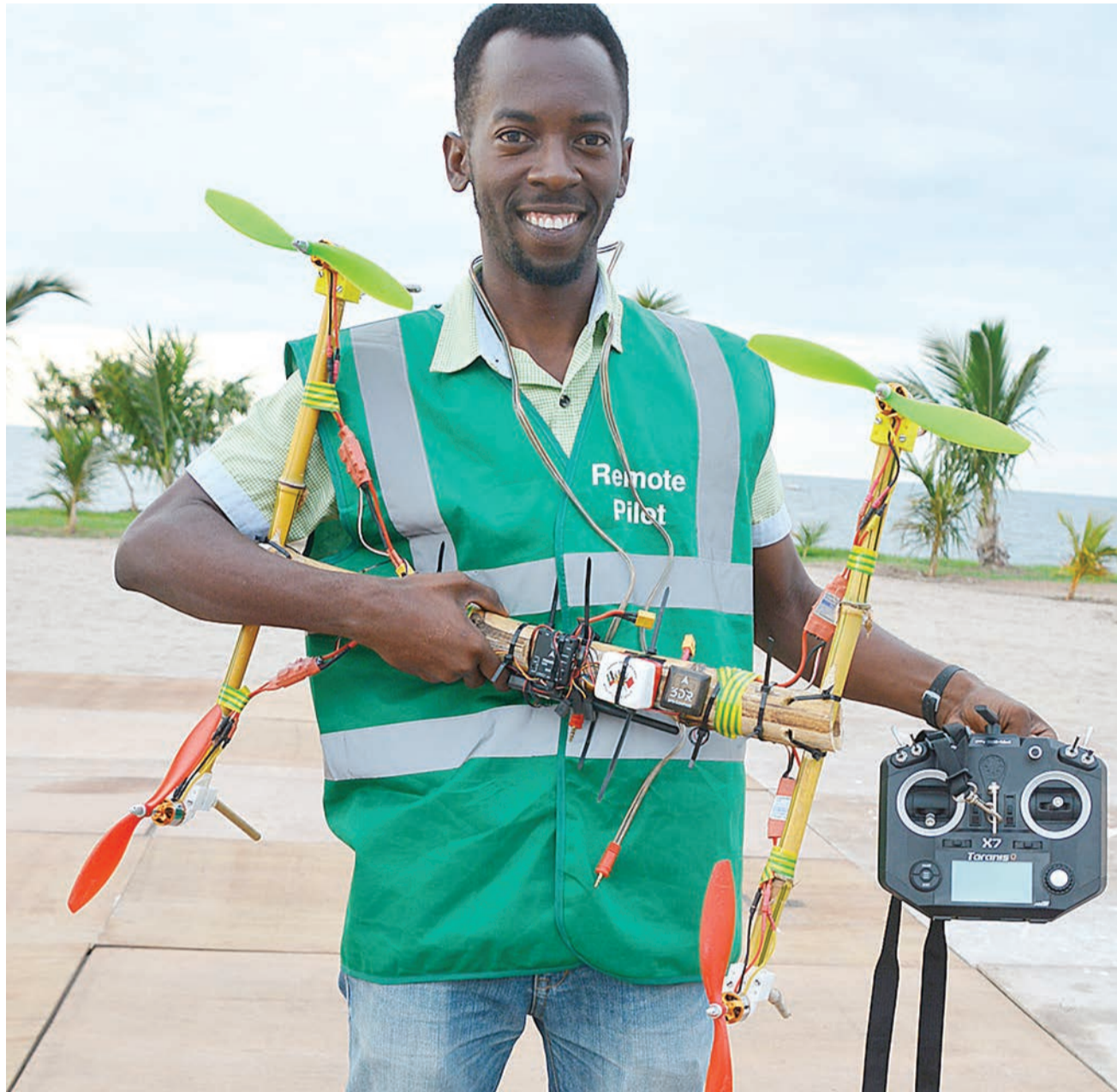
Bornlove Ntikha uses bamboo for the frame of his DIY drone. Ntikha wants to show that drones can be built out of locally available materials, which will make them cheaper and more accessible.
