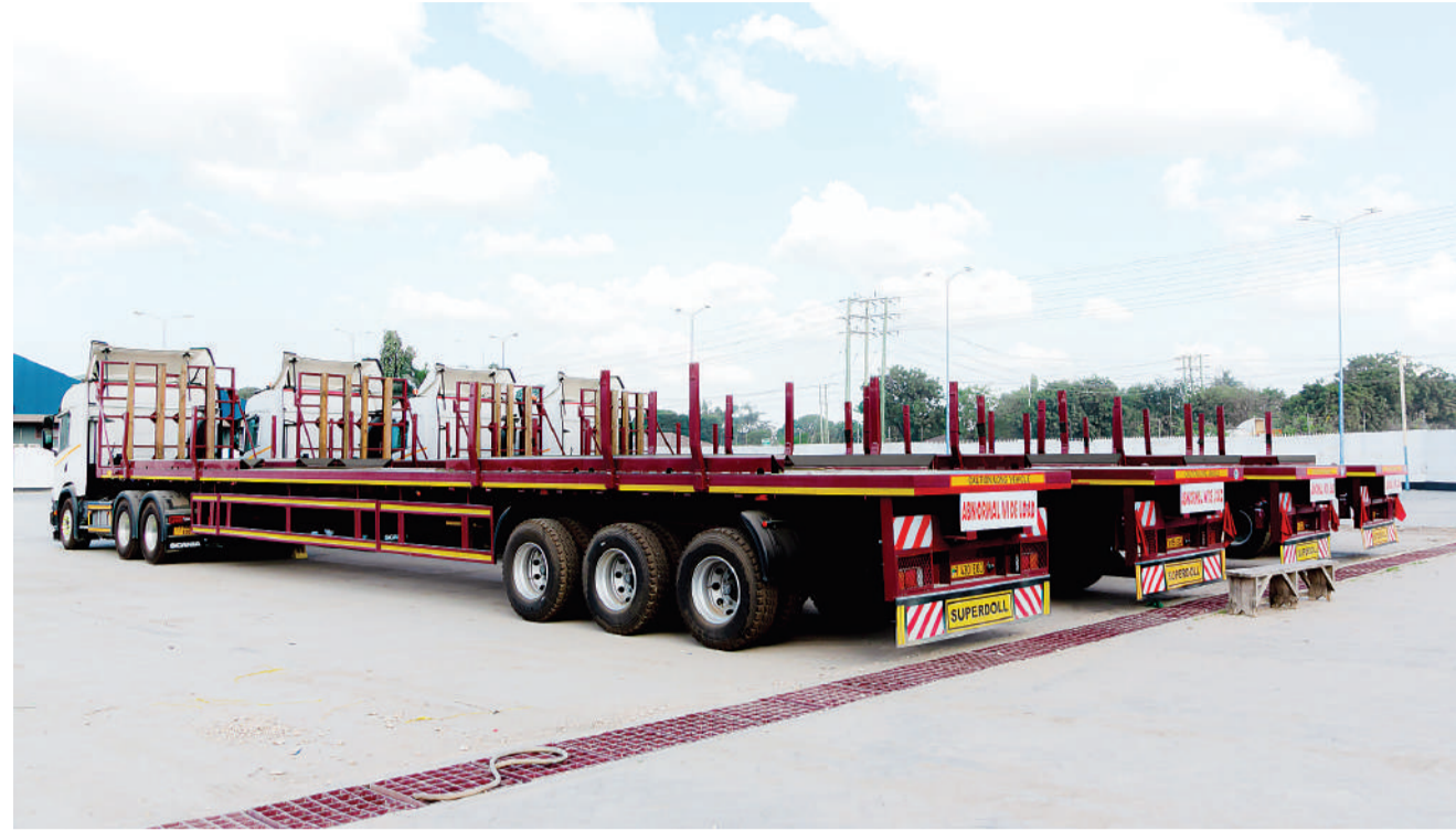
Specialized trailers designed by Superdoll for transporting EACOP pipes
