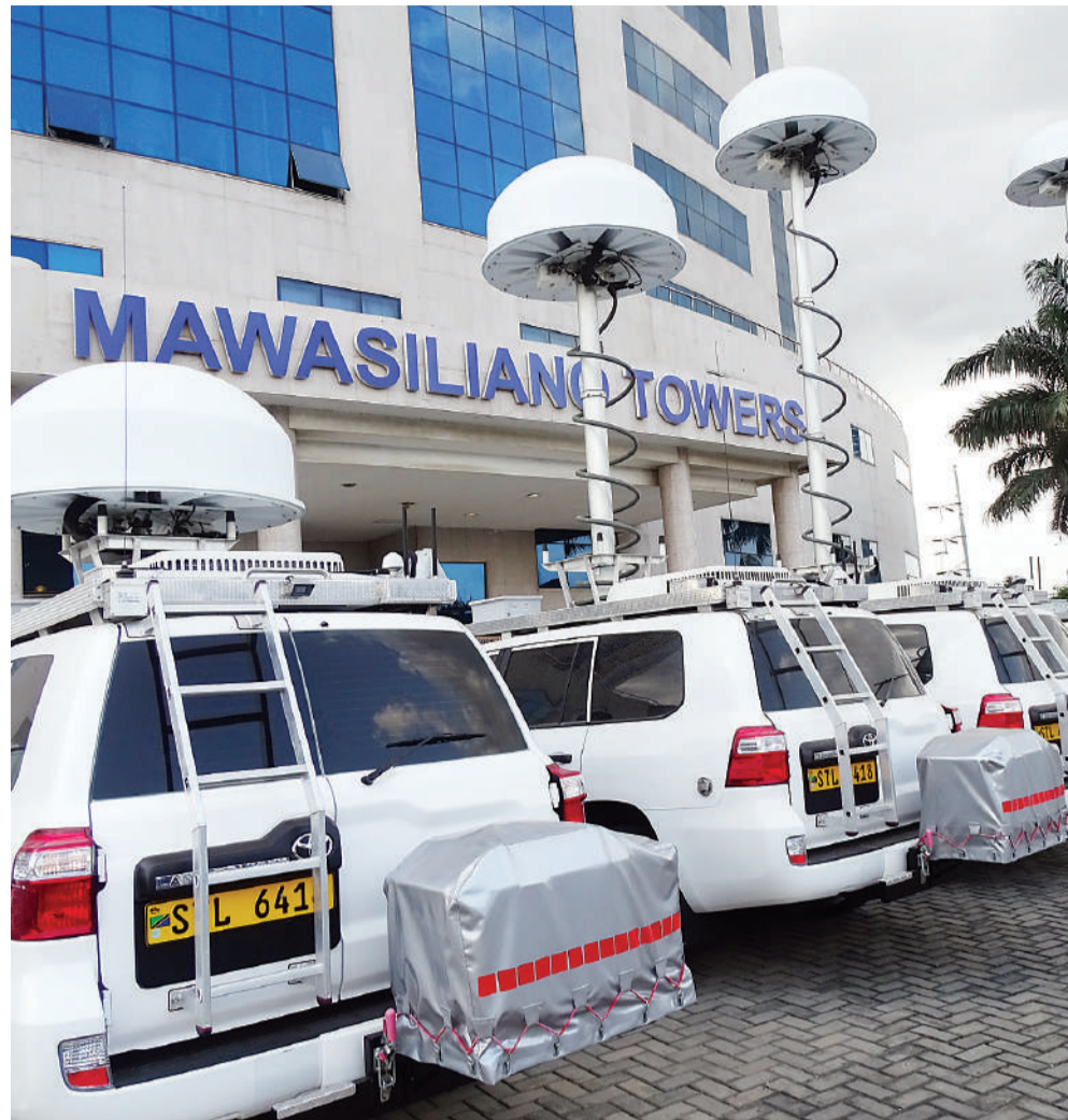
TCRA's recently procured MFMS destined for improved frequency interference mitigation.
