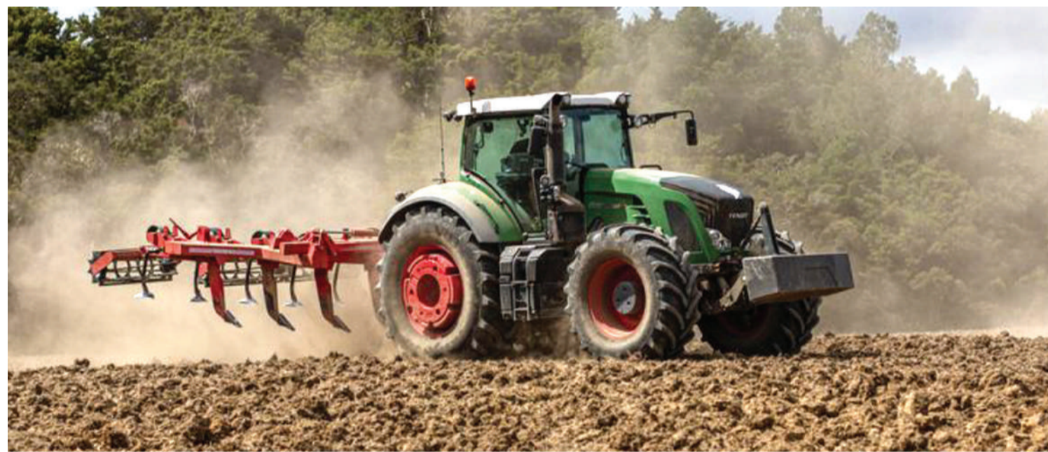
According to the Consultative Group on International Agricultural Research (CGIAR), one of the main benefits of ripping is that can help to break up the hardpan which results from traditional plowing year-after-year, thus improving water infiltration and soil moisture
