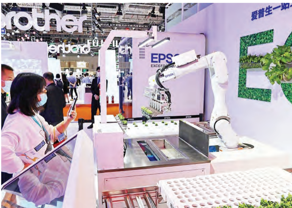
A 6-axis robot developed by Japanese electronics company Seiko Epson Corporation that can screen and grow seedlings attracts visitors at the fourth China International Import Expo in Shanghai, November 2021. (Photo by Xu Congjun/People's Daily Online)
