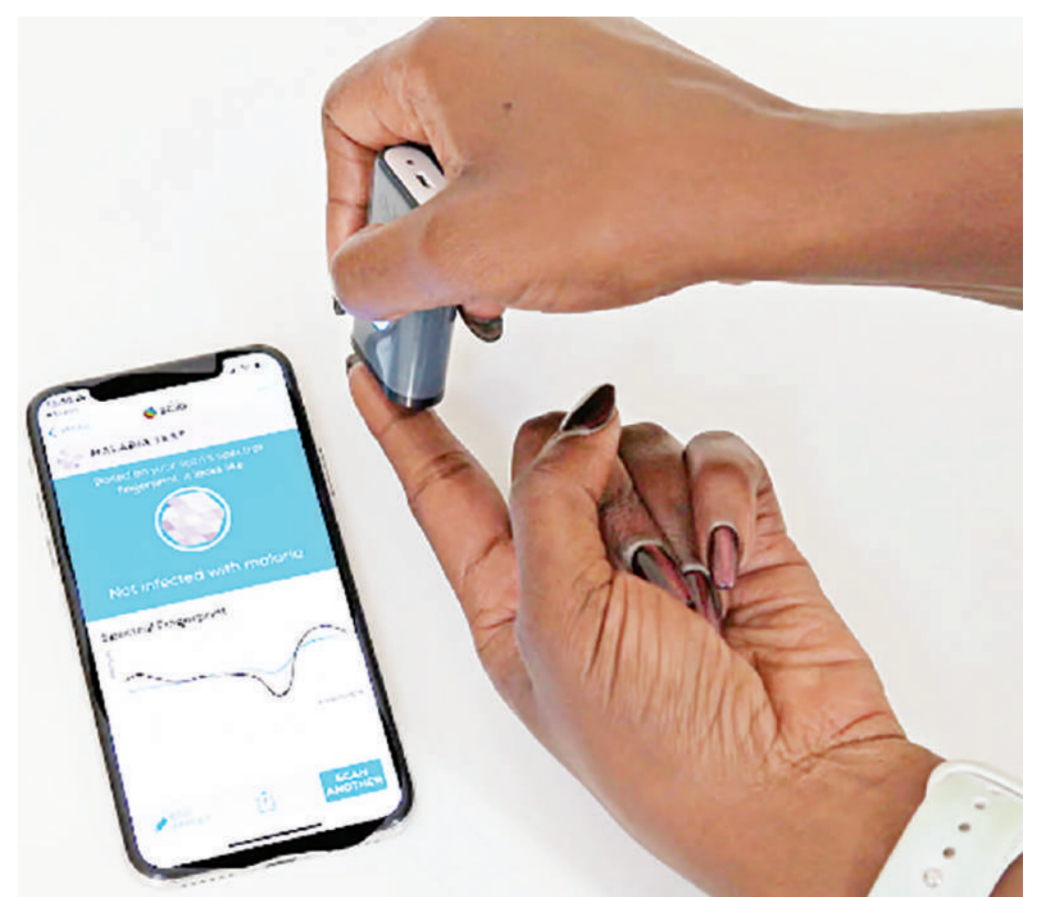
A smartphone-operated spectrometer has been developed to detect changes in blood caused by malaria.
