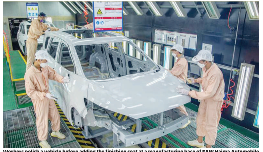
Workers polish a vehicle before adding the finishing coat at a manufacturing base of FAW Haima Automobile Co., Ltd. in Haikou, south China's Hainan province, March 1, 2021. (Photo by Yuan Chen/People's Daily Online)
