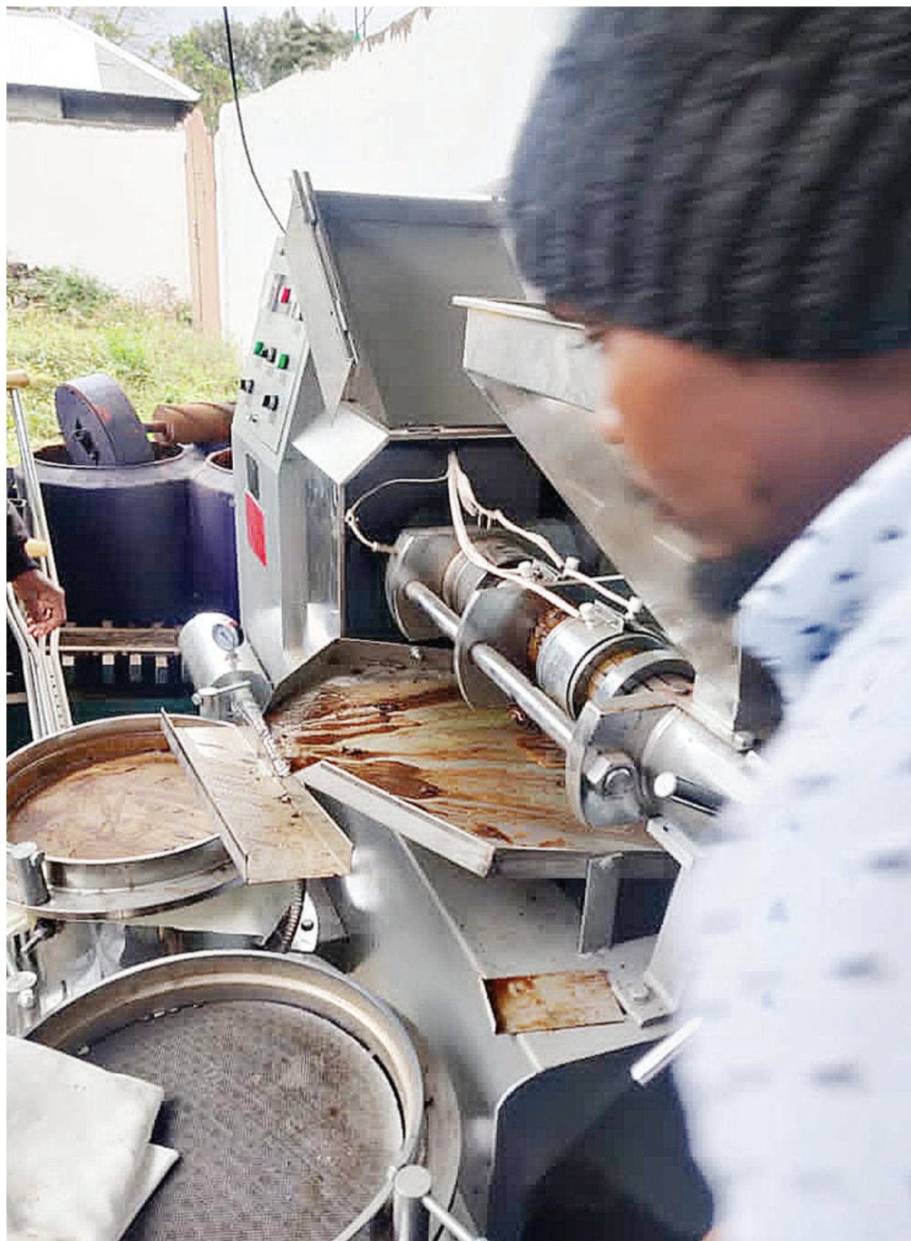
A technician observes the performance of an avocado oil extraction machine. Photo courtesy of Dr Sigisbert Mmasi
