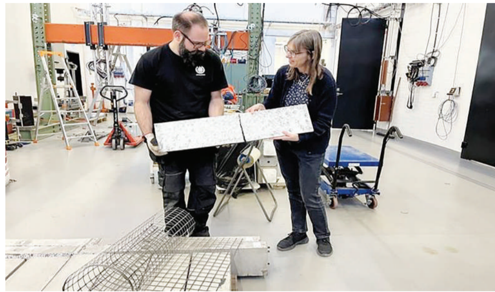
Sebastian Almfeldt (L) and Karin Lundgren, showcase a carbon fiber-reinforced concrete slab. Photo: Mia Halleröd Palmgren/Chalmers
