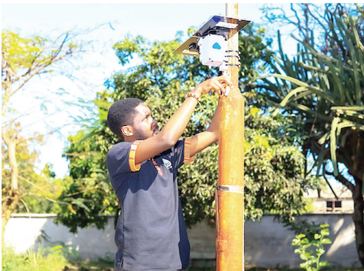
A technician installs a low-cost air quality monitor sensor in Nairobi, Kenya. Air quality monitors are helping Nairobi collect data on air pollution.
