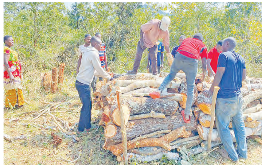
Sustainable charcoal producers in Mapanga village prepare the Improved Basic Earth Mound Kiln (IBEK) for sustainable charcoal production.
