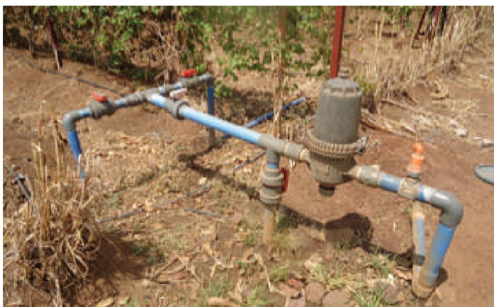
A drip irrigation system implemented in Ikungi, Singida with the support of UN joint programme
