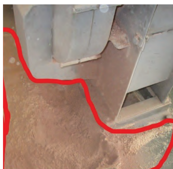
Flour waste (defect) around the milling machine
