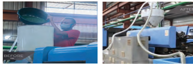
To reduce time consuming through automation. (Left: Before KAIZEN / Right: After KAIZEN)
