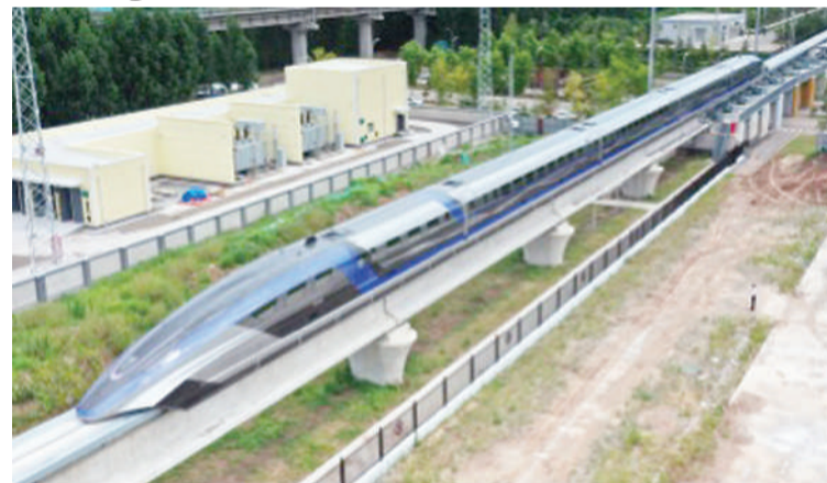
A high-speed maglev train with a designed top speed of 600 kilometers per hour rolls off the production line in Qingdao, east China's Shandong province, July 20, 2021. It is the world's first maglev transportation system that is able to run as fast as 600 kilometers per hour. File photo
