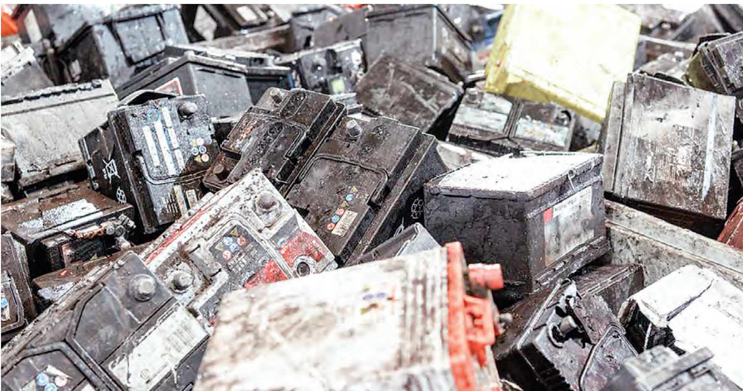
A stockpile of used lead batteries. Inappropriate recycling operations release considerable amounts of lead particles and fumes emitted into the air, deposited onto soil, water bodies and other surfaces with both environmental and human health risks. Photo/ Correspondent Geoffrey Nangai
