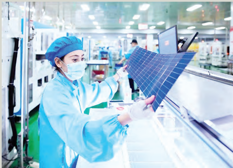
Photovoltaic parts are assembled in a workshop of a solar energy enterprise in Hai'an, east China's Jiangsu province. (People's Daily Online/Zhai Huiyong)
