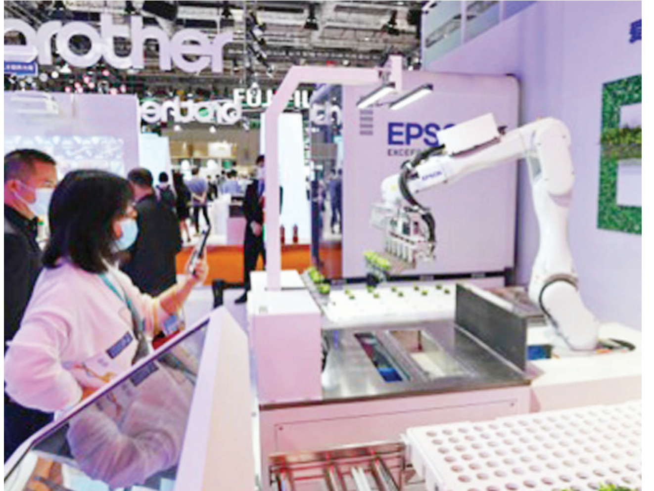
A 6-axis robot developed by Japanese electronics company Seiko Epson Corporation that can screen and grow seedlings attracts visitors at the fourth China International Import Expo held in the National Exhibition and Convention Center (Shanghai) in east China's Shanghai, Nov. 6, 2021. File photo
