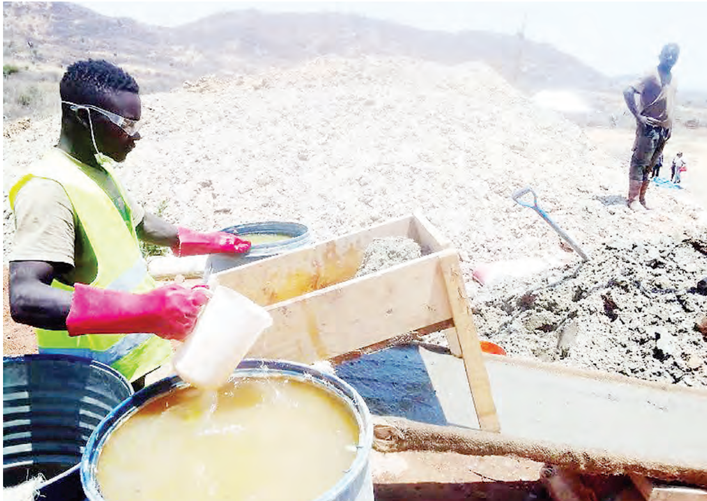
Artisanal miner Aman Mfikwa of Chikoa in Dodoma Region pictured earlier this week using the traditional low-tech way of extracting gold from ore, while wearing protective equipment to minimize the harm the use of mercury can cause. Photo: Correspondent Marco Maduhu
