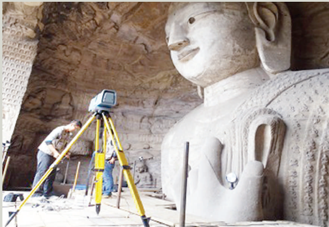
Technicians survey and collect digital images in a cave at the Yungang Grottoes. (Photo from the official website of the Yungang Grottoes)
