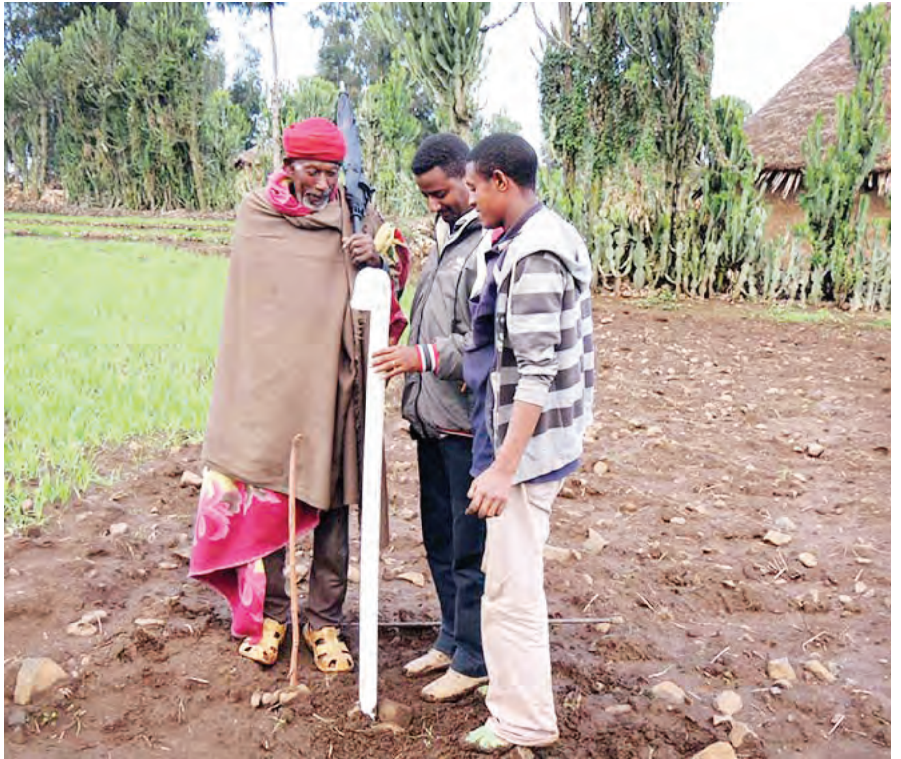
Installing iButton weather sensors in farmers' fields in Tanzania
