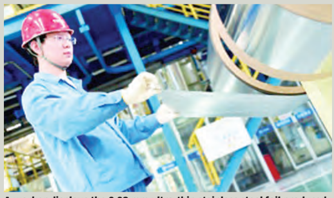
A worker displays the 0.02 mm ultra-thin stainless steel foil produced by Shanxi Taigang Stainless Steel Precision Strip Co., Ltd. (Photo courtesy of Shanxi Taigang Stainless Steel Precision Strip Co., Ltd.)
