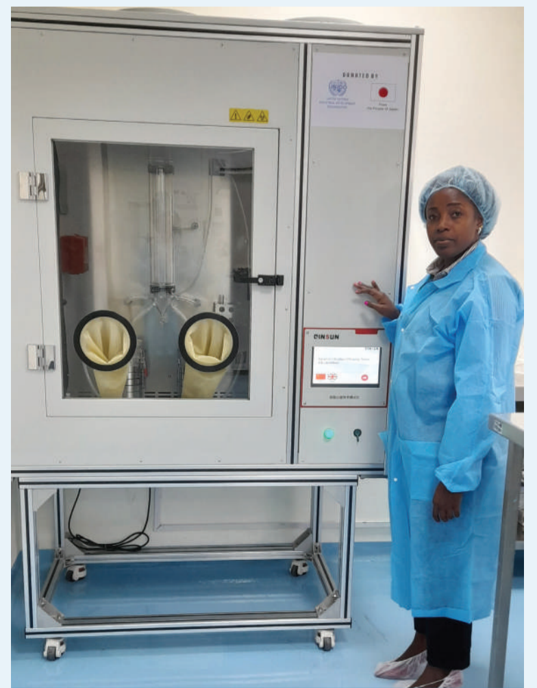
Figure 2: Mask Bacterial Filtration Efficiency Tester
