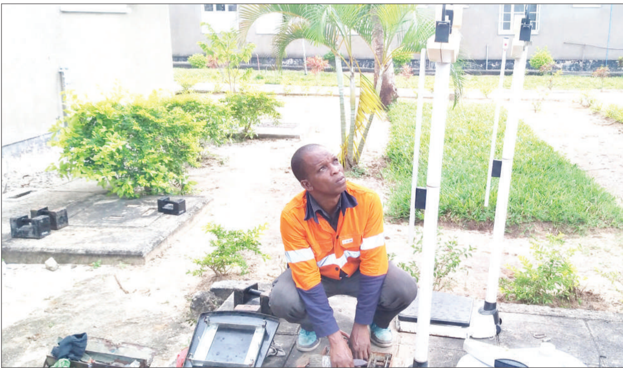
Fundi mizani, Kailan Hussein akirekebisha mzani wa hospitali ya Vijibweni Kigamboni, mkoani Dar es Salaam, wakati Wakala wa Vipimo (WMA), walipotembelea kuhakiki mizani zinazotumika hospitalini hapo jana. PICHA: JOSEPH MWENDA-POLE
