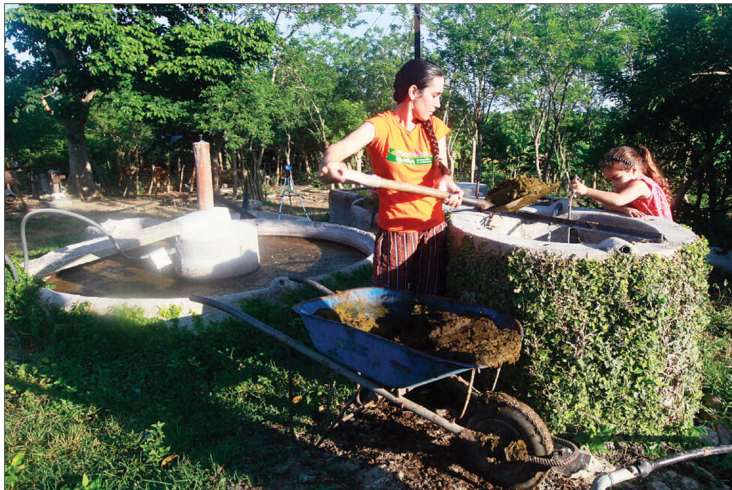
Artist and farmer Chavely Casimiro and her daughter Leah Amanda Diaz feed one of the biodigesters at Finca del Medio, a farm in central Cuba. The biodigester produces about seven meters of biogas per day, enough energy for cooking, baking and dehydrating food. CREDIT: Jorge Luis Baños / IPS
