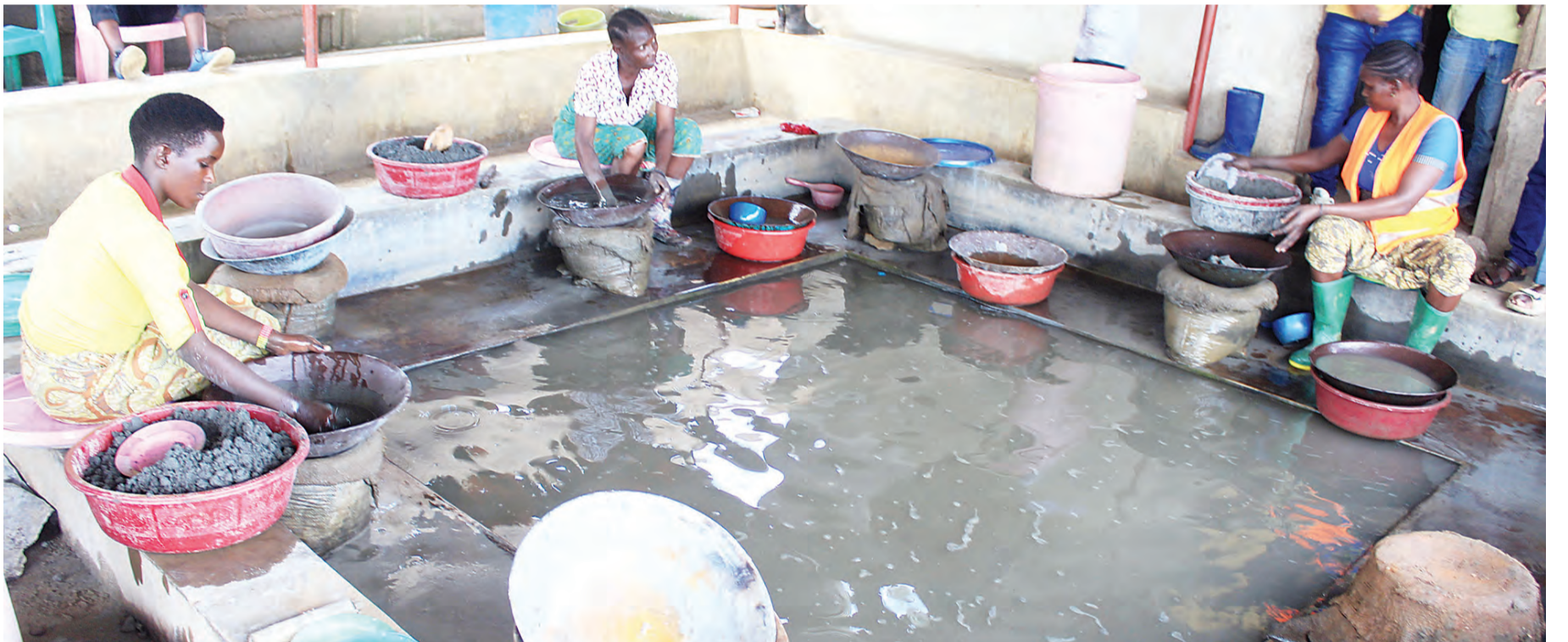
Small-time gold panning in progress at the weekend at the Magunga quarry at Irasanilo artisanal mining site in Butiama District, Mara Region, with mercury heavily in use but with none of those doing the job without any personal protective equipment such as gloves and therefore exposing themselves to health hazards. Photo: Correspondent Marco Maduhu
