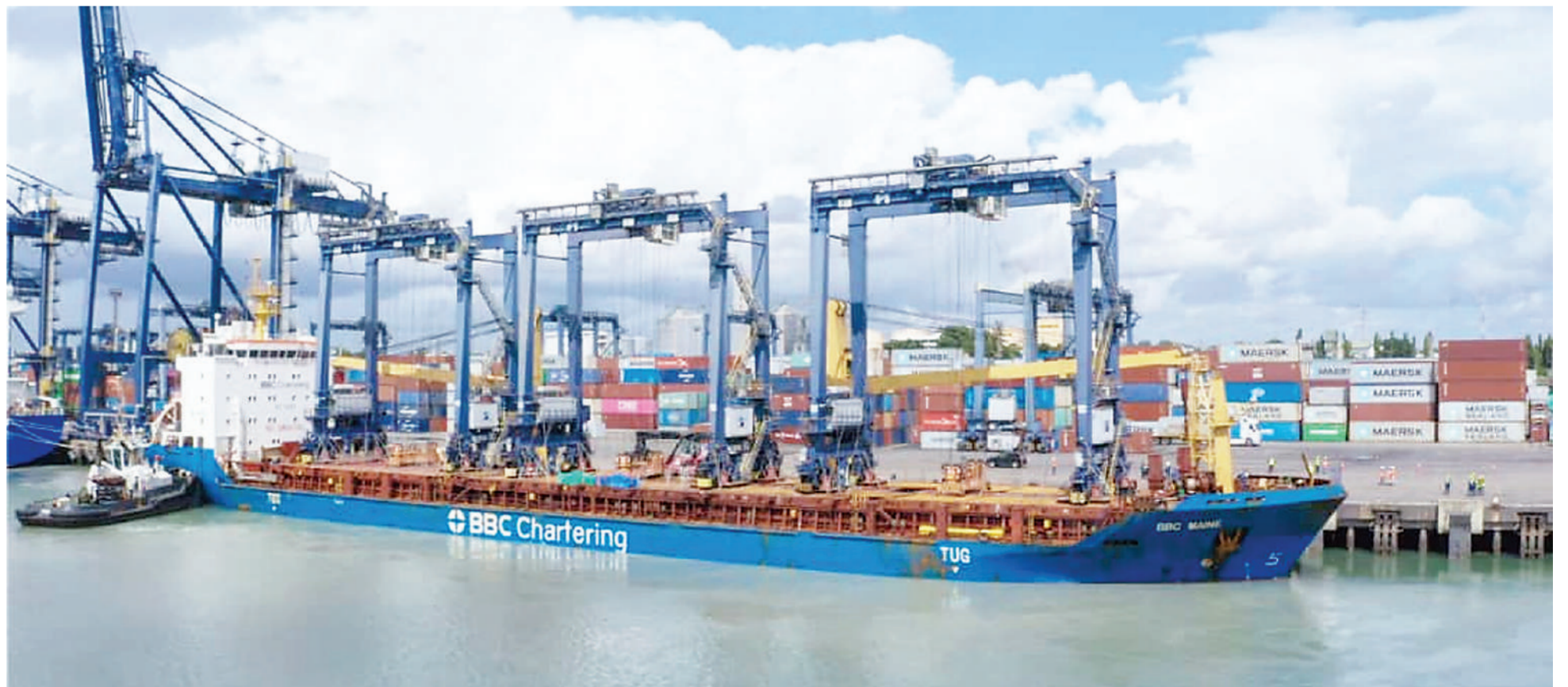
Located at Berths 8 through 11, TICTS operates 725 meters at the port with six quay cranes each with a handling capacity of 45 metric tonnes. With the arrival of the equipment, the terminal current-
