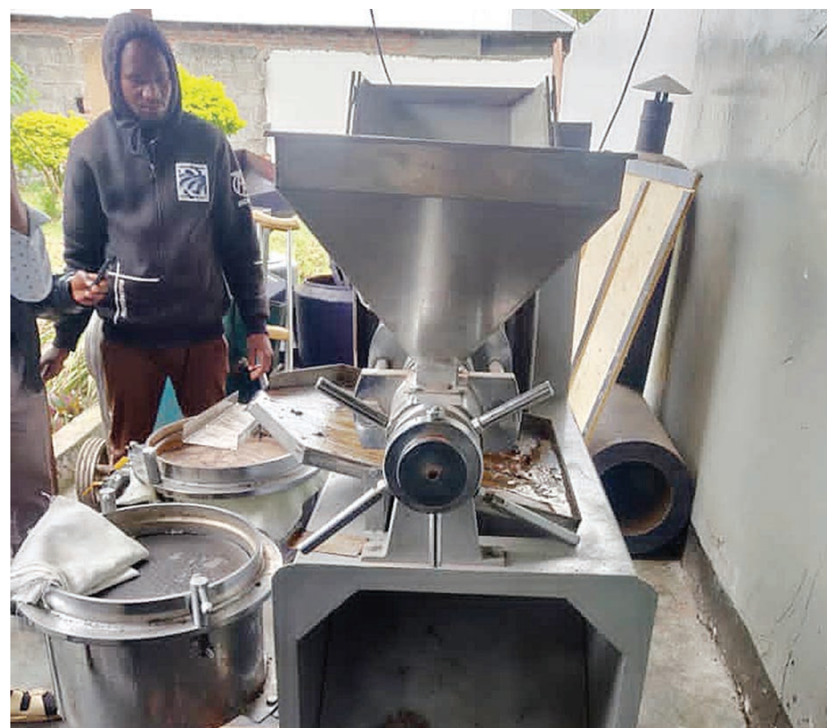
Avocado oil mini-extraction machine designed by TEMDO being tested by technicians to determine the performance of the machine.
