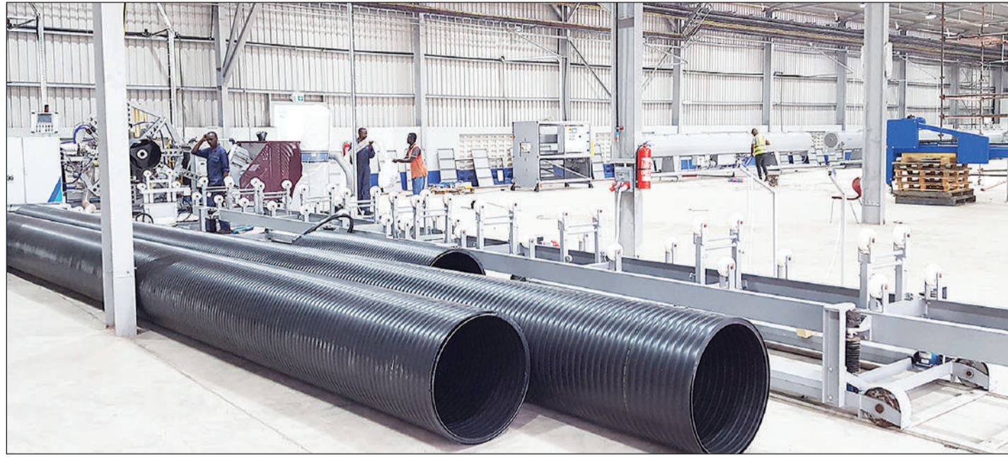
Weholite technology pipes being manufactured at Plasco Limited's factory in Dar es Salaam. File photo
