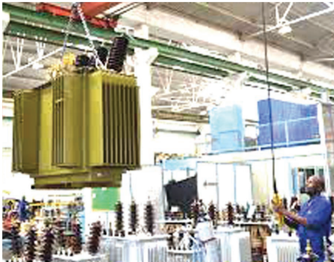
Higher voltage transformers being manufactured by Tanelec Limited at its Arusha factory.
