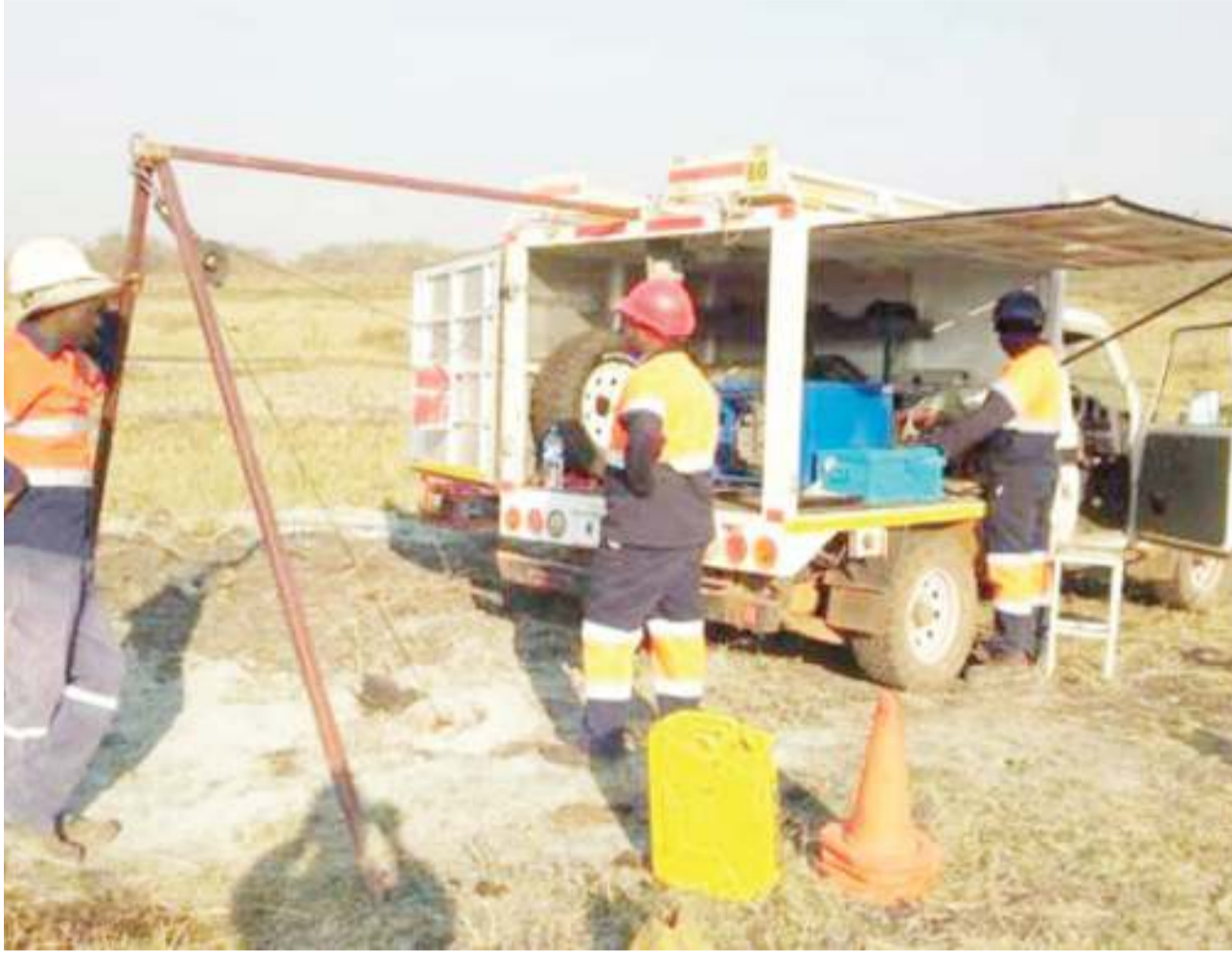
Tanzania Gold Corporation engineers lower a geophysical tool into a drill hole at Buckreef Project in Geita. Photo: TGC website.
