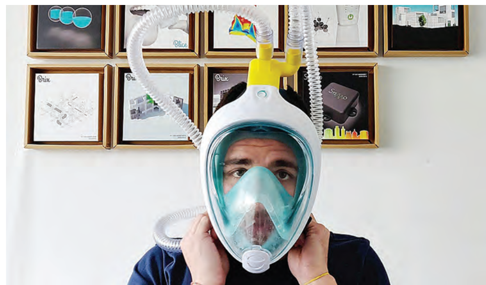
Italian engineering and design start-up Isinnova shows its technical officer Alessandro Romaioli wearing a common snorkelling mask transformed into an emergency respiratory mask with 3D-printed valves.
