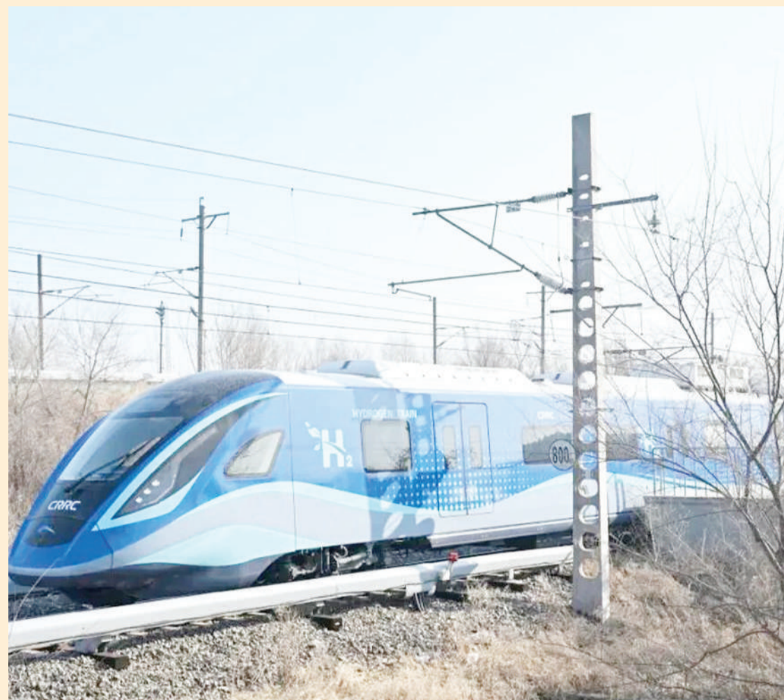
A hydrogen-powered urban train runs on a test track in Changchun, northeast China's Jilin province, March 21, 2024. (Photo courtesy of CRRC Changchun Railway Vehicles Co., Ltd.)
