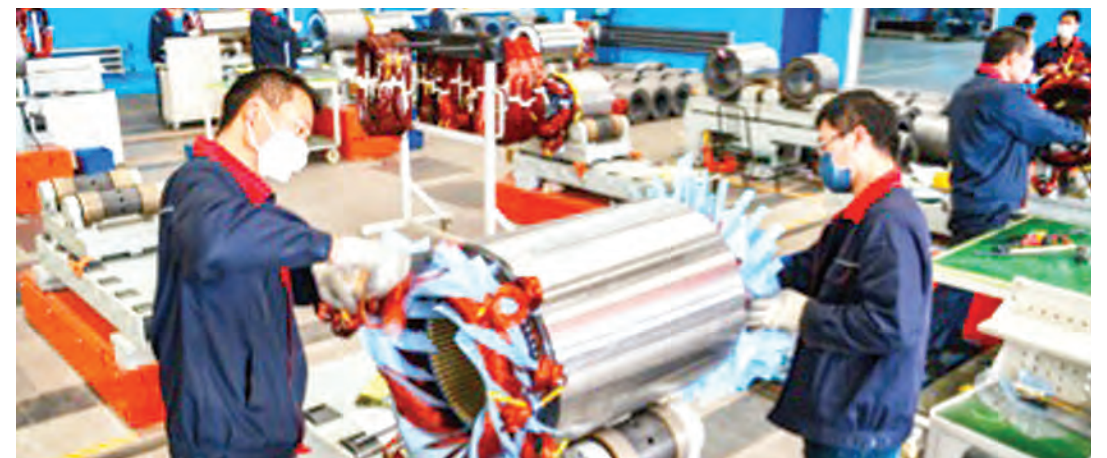
Workers in the large motor workshop of the Hebei large motor workshop at the equipment manufacturing base in Luancheng District, Shijiazhuang City, Hebei Province, are shaping the winding end of the low-voltage high-power motor. Photo: People's Daily
