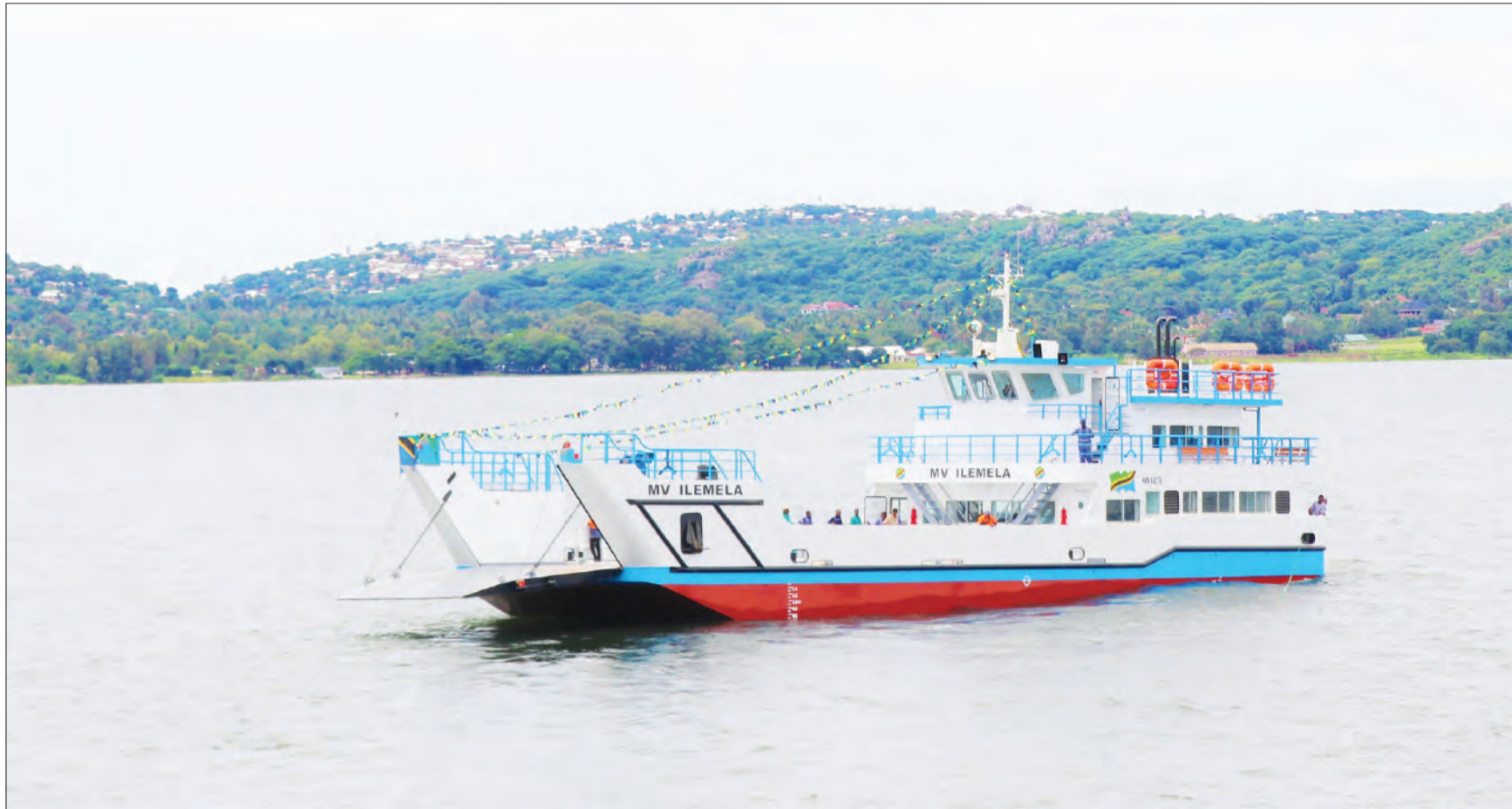
The new pontoon MV. Ilemela floating in the water on Lake Victoria yesterday. It will offer serves between Kayenze and Bezi. It has a seating capacity of 200 passengers and 10 motor vehicles. Photo: Correspondent Alfred Mgweno
